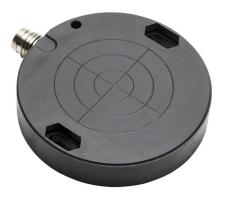
Balluff capacitive proximity sensor, round, 50mm diameter x 10mm body, polyoxymethylene (POM) housing, top sensing, NPN/ PNP, N.O./N.C. selectable, 25mm sensing distance, flush, 50 Hz switching frequency, IP65, 3-pin M8 quick-disconnect.
