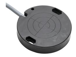
Balluff capacitive proximity sensor, round, 50mm diameter x 10mm body, polyoxymethylene (POM) housing, top sensing, NPN/PNP, N.O./N.C. selectable, 25mm sensing distance, flush, 50 Hz switching frequency, IP67, pigtail.
