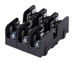
Bussmann modular fuse block, accepts CC fuses, 30A, 600V, 3-pole, 18-10 AWG copper only, pressure plate with quick-connect terminals, 35mm DIN rail or panel mount. Package of 5.
