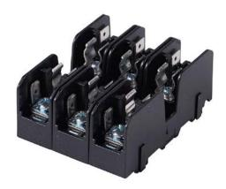
Bussmann modular fuse block, accepts CC fuses, 30A, 600V, 3-pole, 18-10 AWG copper only, pressure plate with quick-connect terminals, 35mm DIN rail or panel mount. Package of 5.
