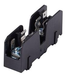
Bussmann modular fuse block, accepts CC fuses, 30A, 600V, 1-pole, 18-10 AWG copper only, pressure plate with quickconnect terminals, 35mm DIN rail or panel mount. Package of 15.
