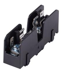
Bussmann modular fuse block, accepts CC fuses, 30A, 600V, 1-pole, 18-10 AWG copper only, pressure plate with quick-connect terminals, 35mm DIN rail or panel mount.
