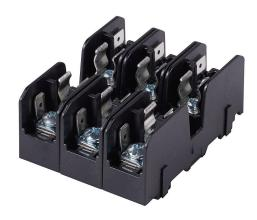
Bussmann modular combination fuse block, accepts (1) Class Midget and (2) Class CC fuses, 30A, 600V, 3-pole, 18-10 AWG copper only, pressure plate with quick-connect terminals, 35mm DIN rail or panel mount. Package of 5.
