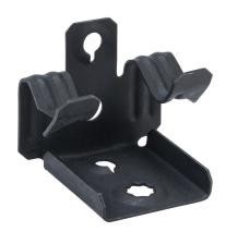
Minerallac hammer-on beam clamp, 75 lbs. Package of 100. For use with 9/16 to 3/4in flanges and 1/4-20 threaded rod.
