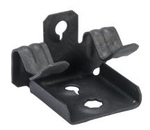
Minerallac hammer-on beam clamp, 75 lbs. Package of 100. For use with 5/16 to 1/2in flanges and 1/4-20 threaded rod.
