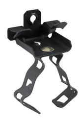
Minerallac hammer-on beam clamp conduit hanger assembly, spring clip, bottom mount, 75 lbs, UL Type UL 2239. Package of 100. For use with 1/8 to 1/4in flanges and 1/2 or 3/4in conduit.
