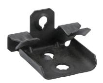
Minerallac hammer-on beam clamp, 75 lbs. Package of 25. For use with 1/8 to 1/4in flanges and 1/4-20 threaded rod.
