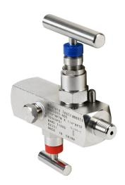
Winters manual block and bleed needle valve, straight body hard seat, double handles, stainless steel body, 1/4in male NPT inlet(s), 1/4in female NPT outlet(s).
