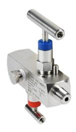
Winters manual block and bleed needle valve, straight body soft seat, double handles, stainless steel body, 1/4in male NPT inlet(s), 1/4in female NPT outlet(s).
