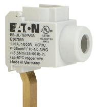
Eaton box type wiring lug, 115A, 1000 VAC/VDC, 1 openings, #10 AWG-1/0 copper only. Package of 3. For use with BBUL series 1-phase busbars.
