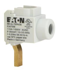
Eaton box type wiring lug, 115A, 1000 VAC/VDC, 1 openings, #10 AWG-1/0 copper only. For use with BBUL series 1-phase busbars.
