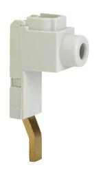
Eaton box type wiring lug, 115A, 1000 VAC/VDC, 1 openings, #10 AWG-1/0 copper only. Package of 3. For use with BBUL series 2-phase and 3-phase busbars.
