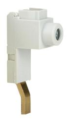
Eaton box type wiring lug, 115A, 1000 VAC/VDC, 1 openings, #10 AWG-1/0 copper only. For use with BBUL series 2-phase and 3-phase busbars.
