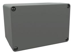
AttaBox BantamBox series enclosure, NEMA 1/3R/4/4X/12, 120 x 80 x 80mm (HxWxD), polycarbonate, RAL 7035 light gray, screw cover, purchase subpanel separately.
