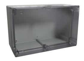
AttaBox BantamBox series enclosure, NEMA 1/3R/4/4X/12, 250 x 160 x 120mm (HxWxD), polycarbonate, RAL 7035 light gray, clear polycarbonate screw cover, purchase subpanel separately.
