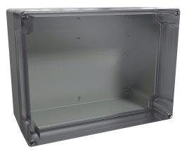
AttaBox BantamBox series enclosure, NEMA 1/3R/4/4X/12, 200 x 150 x 100mm (HxWxD), polycarbonate, RAL 7035 light gray, clear polycarbonate screw cover, purchase subpanel separately.
