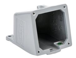
Bryant dead end back box, (1) 1in female NPT conduit entries, cast aluminum housing, gray. For use with Bryant 20A and 30A devices. Requires AP2030 adapter plate.
