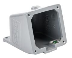
Bryant dead end back box, (1) 3/4in female NPT conduit entries, cast aluminum housing, gray. For use with Bryant 20A and 30A devices. Requires AP2030 adapter plate.
