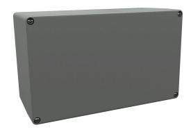
AttaBox BantamBox series enclosure, NEMA 1/3R/4/4X/12, 200 x 120 x 90mm (HxWxD), polycarbonate, RAL 7035 light gray, screw cover, purchase subpanel separately.
