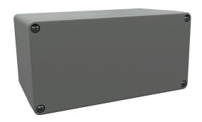
AttaBox BantamBox series enclosure, NEMA 1/3R/4/4X/12,  $160 \times 80 \times 90$ mm (HxWxD), polycarbonate, RAL 7035 light gray, screw cover, purchase subpanel separately.
