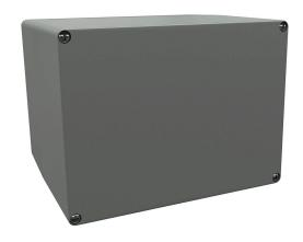
AttaBox BantamBox series enclosure, NEMA 1/3R/4/4X/12,  $160 \times 120 \times 140$ mm (HxWxD), polycarbonate, RAL 7035 light gray, screw cover, purchase subpanel separately.
