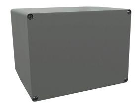
AttaBox BantamBox series enclosure, NEMA 1/3R/4/4X/12, 160 x 120 x 140mm (HxWxD), polycarbonate, RAL 7035 light gray, screw cover, purchase subpanel separately.
