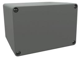
AttaBox BantamBox series enclosure, NEMA 1/3R/4/4X/12, 120 x 80 x 100mm (HxWxD), polycarbonate, RAL 7035 light gray, screw cover, purchase subpanel separately.
