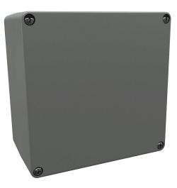
AttaBox BantamBox series enclosure, NEMA 1/3R/4/4X/12, 122 x 120 x 75mm (HxWxD), polycarbonate, RAL 7035 light gray, screw cover, purchase subpanel separately.
