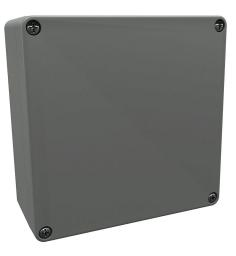
AttaBox BantamBox series enclosure, NEMA 1/3R/4/4X/12, 122 x 120 x 55mm (HxWxD), polycarbonate, RAL 7035 light gray, screw cover, purchase subpanel separately.
