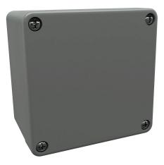
AttaBox BantamBox series enclosure, NEMA 1/3R/4/4X/12, 82 x 80 x 55mm (HxWxD), polycarbonate, RAL 7035 light gray, screw cover, purchase subpanel separately.
