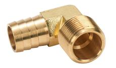
NITRA water, oil, air or gases threaded fitting, hose barb elbow, brass body, brass threads, (1) 3/4in male NPT to (1) 3/4in hose. Package of 3.
