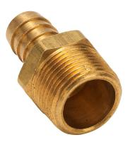
NITRA water, oil, air or gases threaded fitting, hose barb, brass body, brass threads, (1) 3/4in male NPT to (1) 5/8in hose. Package of 3.
