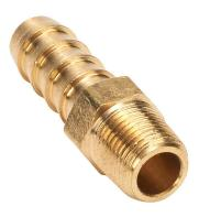
NITRA water, oil, air or gases threaded fitting, hose barb, brass body, brass threads, (1) 1/8in male NPT to (1) 5/16in hose. Package of 5.
