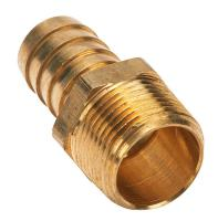
NITRA water, oil, air or gases threaded fitting, hose barb, brass body, brass threads, (1) 3/4in male NPT to (1) 3/4in hose. Package of 3.
