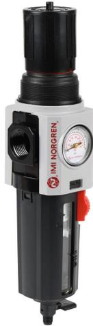
Norgren Excelon Plus 84 pneumatic filter-regulator, 3/4in female NPT inlet(s), 3/4in female NPT outlet(s), 4-145 psi range, manual drain, polycarbonate bowl, bowl guard. For use with Excelon 84 series components.
