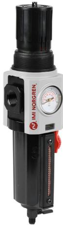
Norgren Excelon Plus 84 pneumatic filter-regulator, 1/2in female NPT inlet(s), 1/2in female NPT outlet(s), 4-145 psi range, manual drain, die-cast aluminum bowl, sight gauge. For use with Excelon 84 series components.
