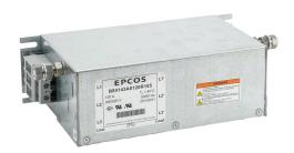
AutomationDirect EMI input filter, 480 VAC, 3-phase, 120A, panel mount, EMI/RFI filtering, drive rated, standard performance, screw terminals and ring terminals. For use with 3-phase GS30 series frame G AC drives.
