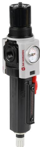
Norgren Excelon Plus 82 pneumatic filter-regulator, 1/4in female NPT inlet(s), 1/4in female NPT outlet(s), 4-145 psi range, automatic drain, die-cast zinc bowl, sight gauge. For use with Excelon 82 series components.
