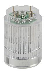
Patlite LED light element, 25mm diameter, yellow, permanent light function, 24 VDC, NPN polarity, clear lens. For use with ME and MES series signal towers.
