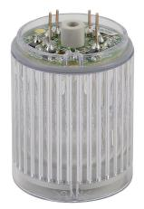
Patlite LED light element, 30mm diameter, yellow, permanent light function, 24 VAC/VDC, clear lens. For use with MP and MPS series signal towers.
