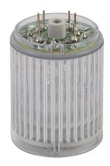
Patlite LED light element, 30mm diameter, clear/white, permanent light function, 24 VAC/VDC, clear lens. For use with MP and MPS series signal towers.
