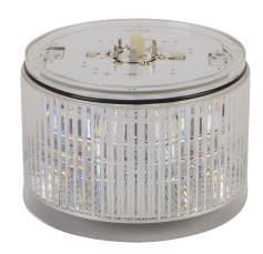
Patlite LED light element, 100mm diameter, clear/white, permanent or flashing (60 fpm +/- 3 fpm) light function, 24 VDC, clear lens. For use with LKEH series signal towers.
