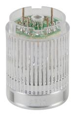
Patlite LED light element, 25mm diameter, blue, permanent light function, 24 VDC, PNP polarity, clear lens. For use with ME and MES series signal towers.
