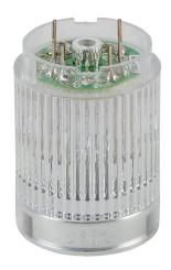
Patlite LED light element, 25mm diameter, green, permanent light function, 24 VDC, PNP polarity, clear lens. For use with ME and MES series signal towers.
