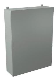
Wiegmann enclosure, NEMA 12, 48 x 36 x 11in (HxWxD), wall mount, carbon steel, ANSI 61 gray, powder coat finish, single-door, (4) plated steel clamps.
