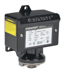
Ashcroft mechanical pressure switch, 9 to 60 psig set point, 1.4 to 4.9 psig deadband range, Viton sensing element, Viton seal(s), SPDT 15A, 1/4in female NPT process connection, 3/4in female NPT conduit opening.
