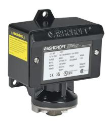
Ashcroft mechanical pressure switch, 60 to 400 psig set point, 7.0 to 33.6 psig deadband range, Viton sensing element, Viton seal(s), SPDT 15A, 1/4in female NPT process connection, 3/4in female NPT conduit opening.
