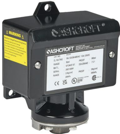
Ashcroft mechanical pressure switch, 4.5 to 30 psig set point, 0.7 to 2.1 psig deadband range, Viton sensing element, Viton seal(s), SPDT 15A, 1/4in female NPT process connection, 3/4in female NPT conduit opening.
