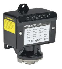
Ashcroft mechanical pressure switch, 30 to 200 psig set point, 7.0 to 18.2 psig deadband range, Viton sensing element, Viton seal(s), SPDT 15A, 1/4in female NPT process connection, 3/4in female NPT conduit opening.
