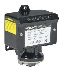
Ashcroft mechanical pressure switch, 15 to 100 psig set point, 2.1 to 7.0 psig deadband range, Viton sensing element, Viton seal(s), SPDT 15A, 1/4in female NPT process connection, 3/4in female NPT conduit opening.
