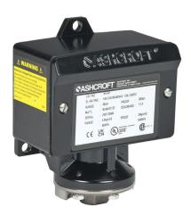
Ashcroft mechanical pressure switch, 9 to 60 psig set point, 1.0 to 3.5 psig deadband range, Buna-N sensing element, Buna-N seal(s), SPDT 15A, 1/4in female NPT process connection, 3/4in female NPT conduit opening.
