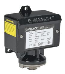
Ashcroft mechanical pressure switch, 60 to 400 psig set point, 5 to 24 psig deadband range, Buna-N sensing element, Buna-N seal(s), SPDT 15A, 1/4in female NPT process connection, 3/4in female NPT conduit opening.
